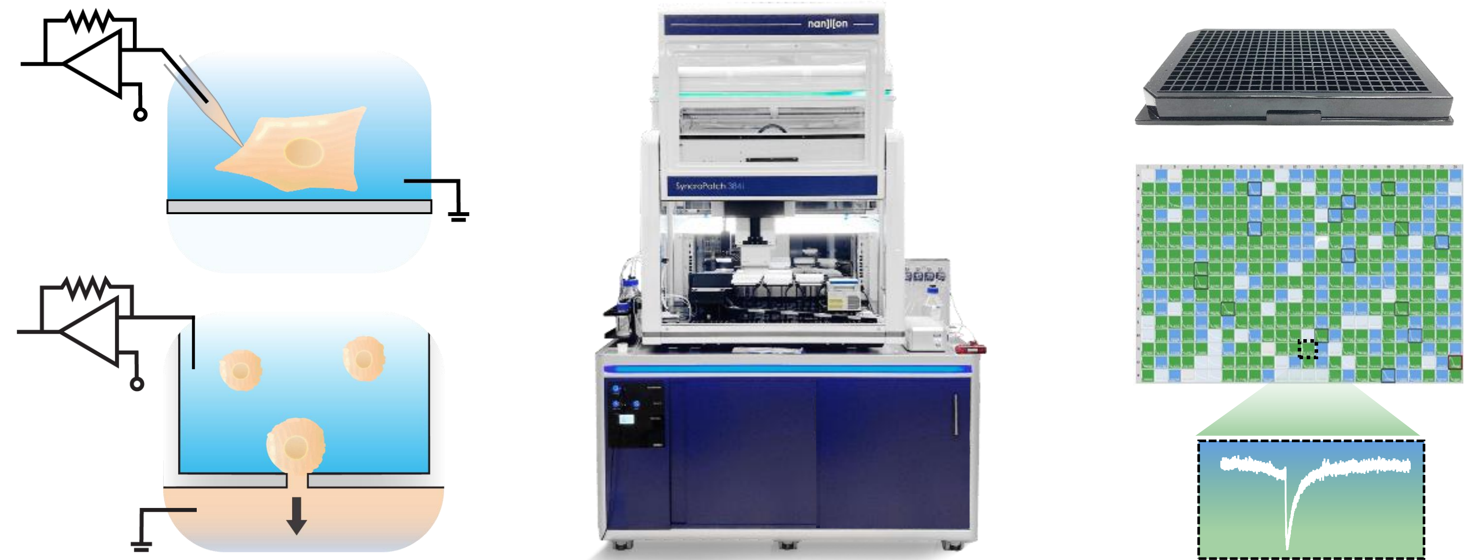
Figure 1. Automated Patch Clamp (APC) overview. A, Traditional patch clamp (upper) and fixed-well APC (lower). B, Syncropatch 384. C, Consumable 384-well chip (upper) with a software screenshot during an example experiment with a representative trace highlighted (lower).
