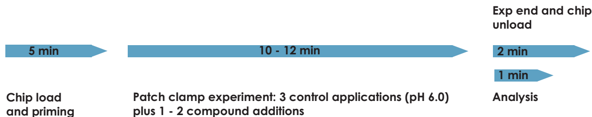
Figure 6: Timeline of an experiment on the SyncroPatch 384PE. The completion of 1 experiment on the SyncroPatch® 384 patch clamp chip (384 wells) for a single point concentration response curve on ASIC3-mediated currents took approximately 17-19 min.
